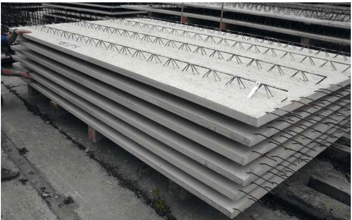
► FIG. 3 Factory-produced prototype precast floor slabs (by Beton Kemmler GmbH) consisting of "eco-concrete" with reduced cement content. //
