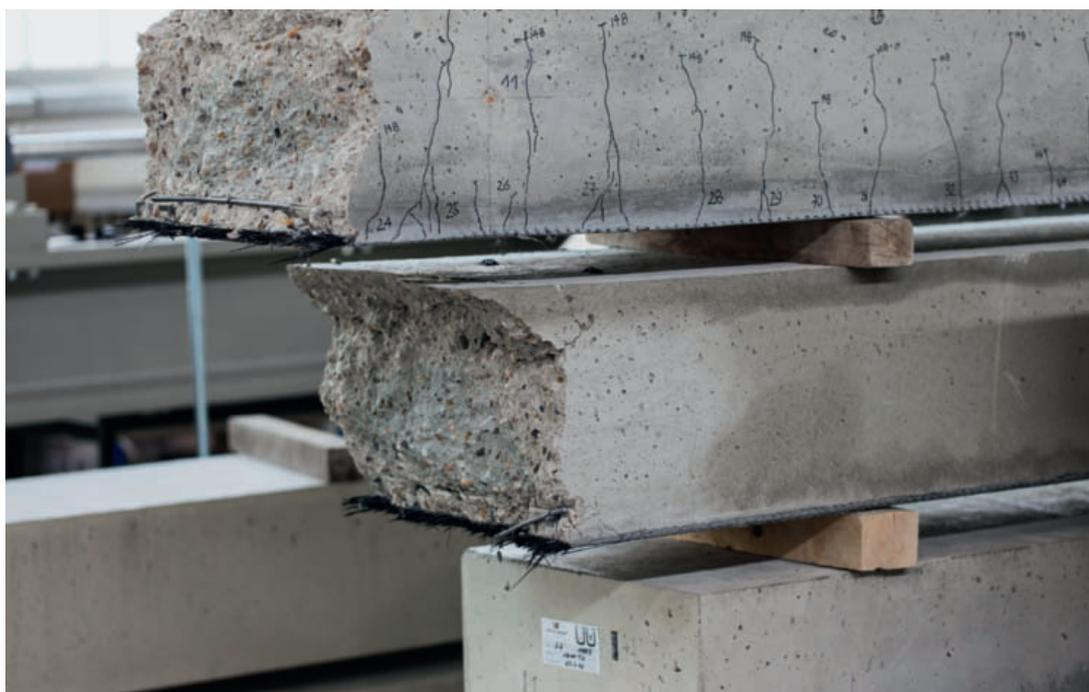
→ Textile-reinforced structural concrete slab after testing (tensile failure of textile) [3]
