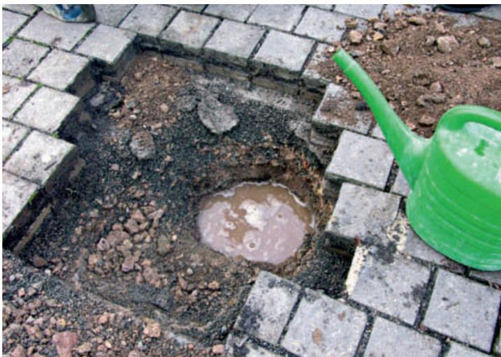
→ 1 Insufficient permeability of the structural layer
