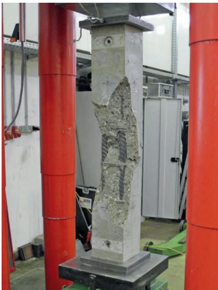
→ 2 Column with longitudinal reinforcement of  $\varnothing 40$  mm after the test
