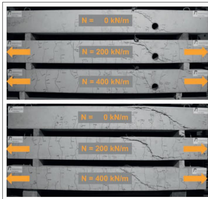
→ 1 Example of the regular longitudinal tensile forces in the test bench for a test series
