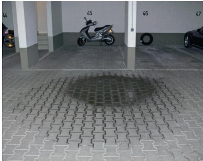
→ 1 Spread of 10 l of water after 10 minutes on a block pavement
