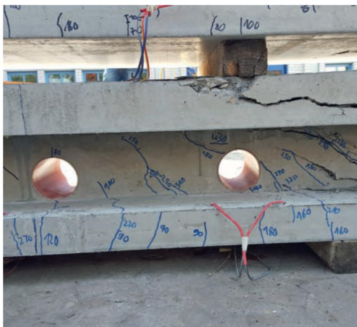
→ Tests performed on the assembled slabs with sandwich cross section
